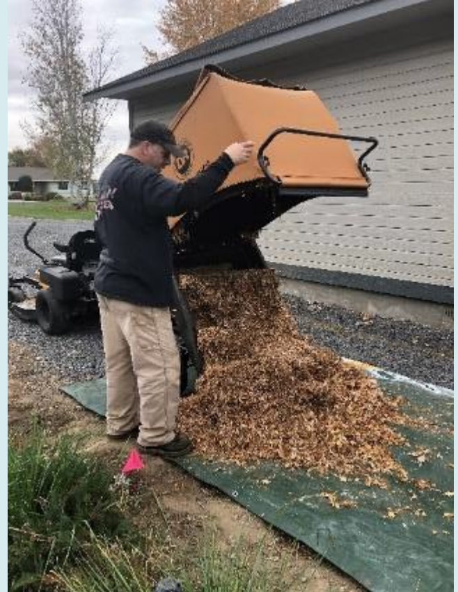
This leaf catcher is pulled behind a lawn mower that picks up and shreds them for easy removal.
